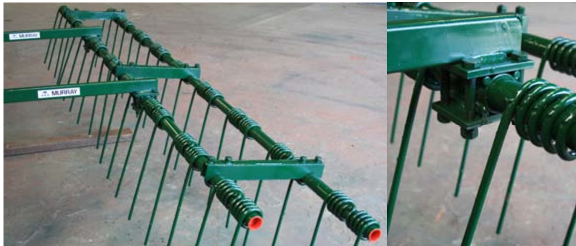
Series 30 Model 30008 3.20m (10'6") 2 Rank Spring Tine shown
