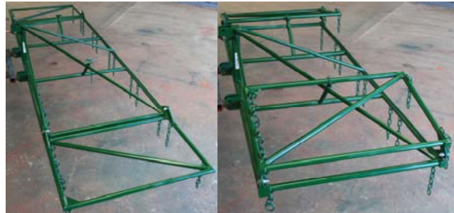
Series 38 Model 38009, 3 Point Linkage Folding Wing Harrow Frame shown – Open & Closed
